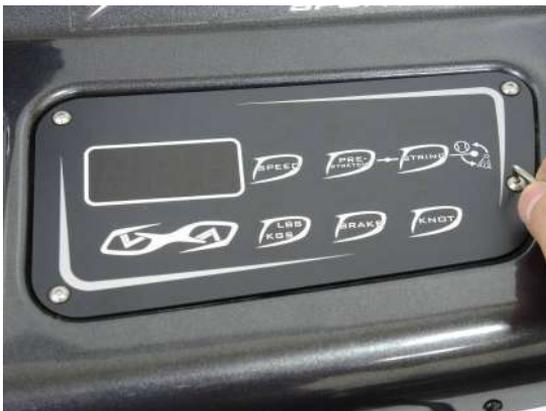
Using a 2.5mm L-shape allen wrench to loosen the 4 screws on the control panel and lift the right side of control panel
