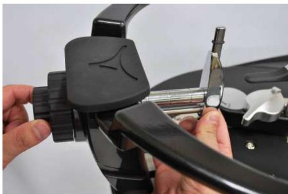
Insert the badminton L shape main pins in the frame support posts.
