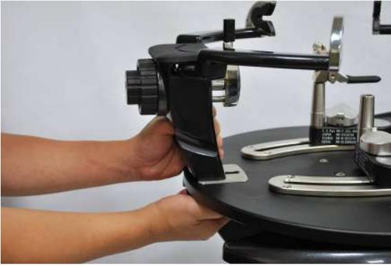
Adjust the frame support posts to the proper position according to the racquet frame.
