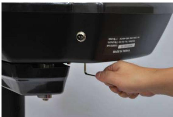
Fix the drawer on the machine base by using 4mm allen wrench to tighten the 2 screws (SOM5x12).
