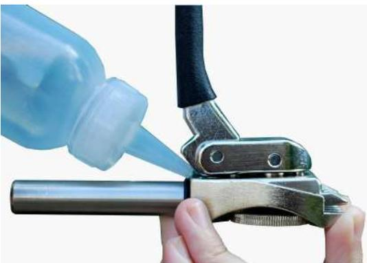
The contact surface of the string clamp handles receive a lot of compression while locking and unlocking clamp; therefore it is recommended to use Teflon based oil to keep this part well lubricated.
