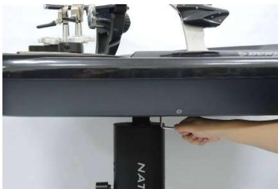
Fix the machine top on the stand set by using 6mm allen wrench to tighten the 4 screws (SOM8x20).
