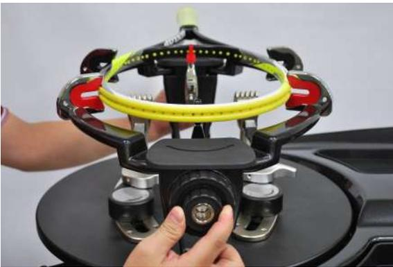
Adjust the small knobs to let the frame pad of main pin touch racquet.
