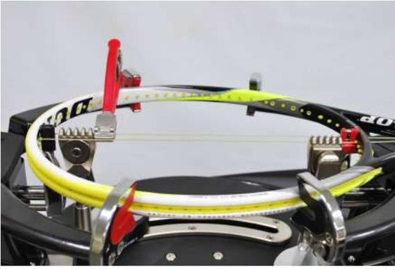
Clamp a start clamp as close to the clamp as possible.
