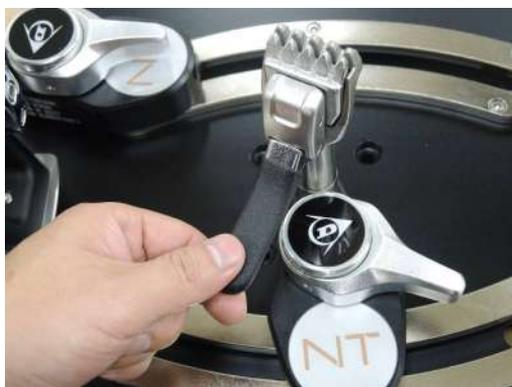
Open the clamp handle and let it fall down can release the clam base at the same time.
