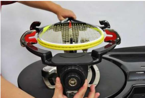
Then loosen the mounting arms by turning the big knob. Thus allowing you to take the strung racquet from mount system easily.
