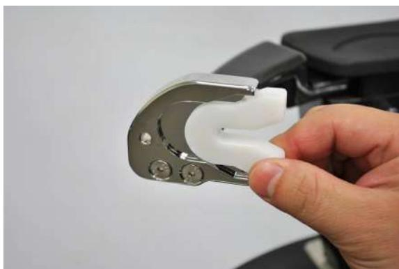
Insert the badminton frame support pads in the frame supports.
