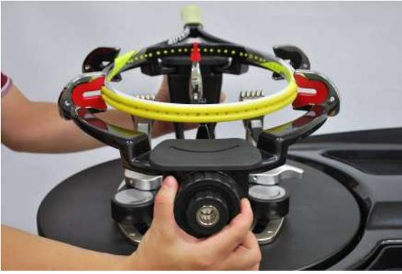
Double check the 2 big knobs if tighten.
