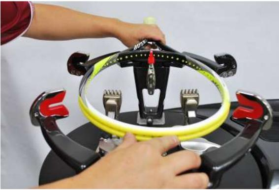
Place the frame at the middle of mounting system.
