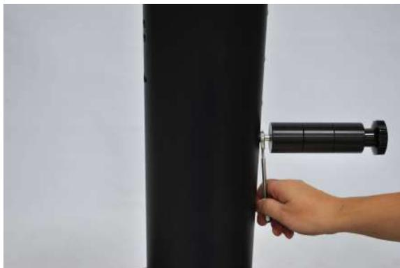
Use 13 mm Box & Open End Wrench to tighten string reel hanger .
