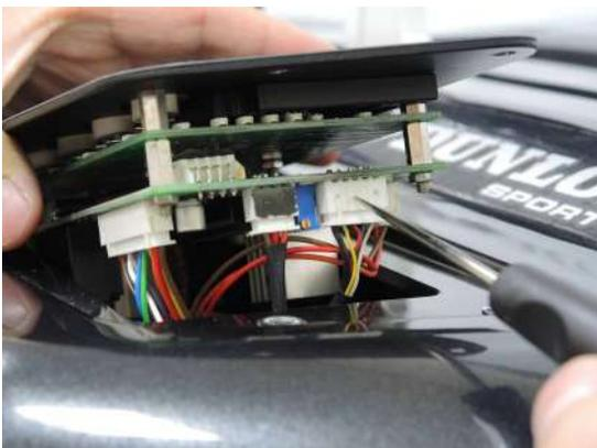
Check the wire connection of sensor for the E01 error.
