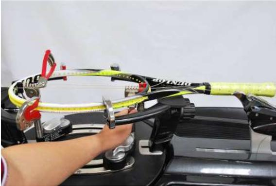
Tension the first string again. Release the string clamp and clamp again while tensioning. This step is for retrieve the tension loose.
