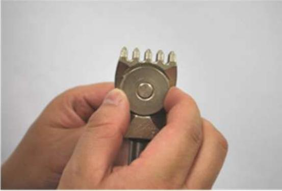
In order to avoid string damage, adjust the string clamps pressure to eliminate string slippage and avoid over tightening before you start stringing.
