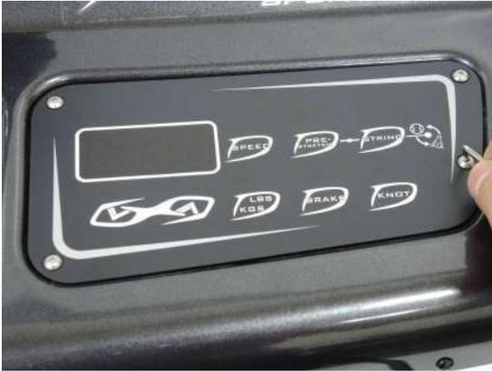
Using a 2.5mm L-shape allen wrench to loosen the 4 screws on the control panel and lift the right side of control panel will find the fine adjustment knob of tension adjusting.
