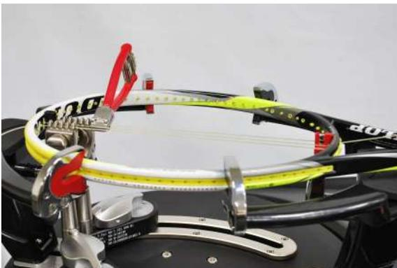
Pull the other string which is clamped by start clamp.
