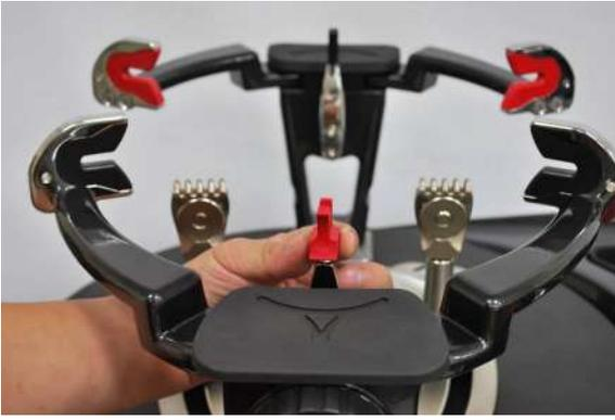
Insert the proper frame pads on the main pins.
