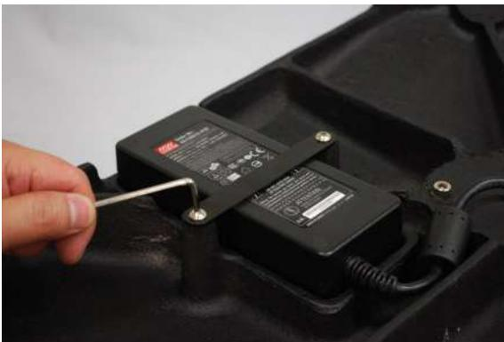
Put the adapter in the groove of foot. Tighten the fixed bar of the adapter with the foot by 3mm allen wrench.
