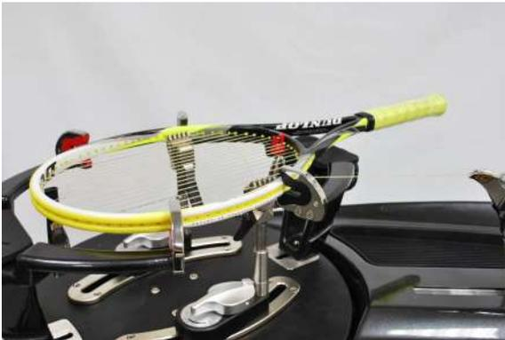
Press the “KNOT” button to increase 10% of setting tension before pulling the last main string.
