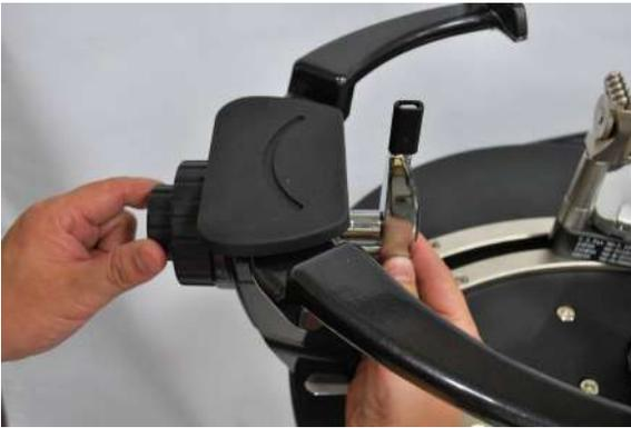
Insert the tennis L shape main pins in the frame support posts.
