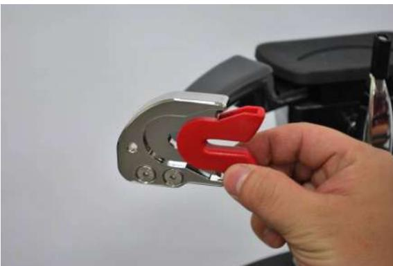
Insert the tennis frame support pads of tip side in the frame supports.
