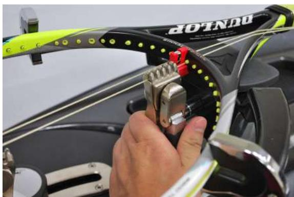
Move clamp base to the appropriate position and clamp one of string.
