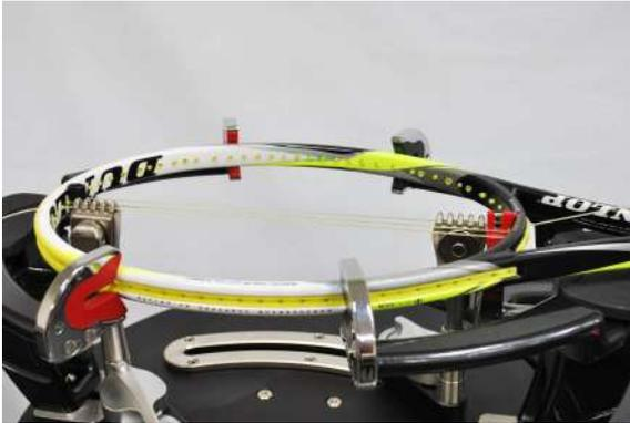
Clamp the string which is close to the tensioning side again.
