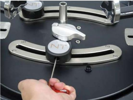
When the clamp base locking lever had been well locked but still feel some slight movement on the base, please use a 3mm T- wrench to fine tune the screw as shown. Turn it clockwise to tighten the base, avoid excessive turning to cause the Base moving difficult.
